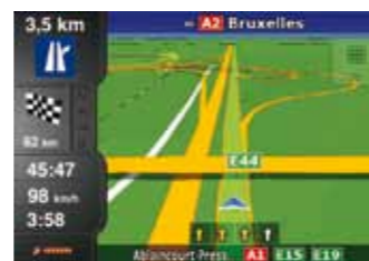
Automatic smart zoom function to enlarge intersections and turning lanes
