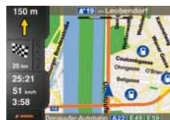
In 2-D mode the map orientation can be set to north or else, aligned with the direction of driving.
