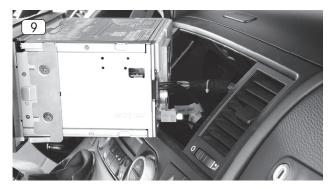
9. Connect all the cables to the ZENEC system (No. 1) those previously run in the radio slot, and the original antenna cables.
