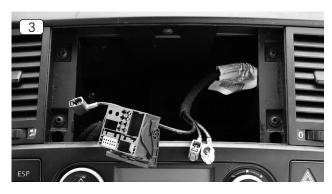
To completely remove the factory radio, all the cables (i.e. main wire harness, antenna cable etc.) must be unplugged on the backside of the device. Put the radio aside in a safe place, to protect it from damage.
