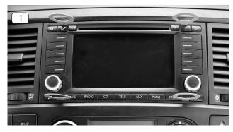
Unlock the OE factory radio with the unlock tool (No. 10) contained in the set. You need to insert all four keys.
