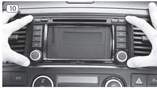
Neatly arrange the wires to the side, making room for the ZENEC system. Carefully slide it into the radio slot. Push back the Z-E2060 until you hear the clicking sound of the latching mechanism.
