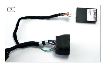
Connect one of the main connection cables (No. 4) of the ZENEC system (No. 1) to the Quadlock connector of the car and close its locking mechanism. Following this, connect the CAN bus interface (No. 5) to the main connection cable.
