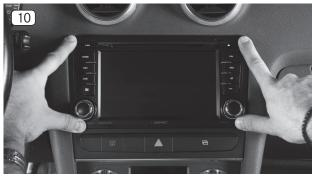
Neatly arrange the wires to the side, making room for the ZENEC system. Carefully slide it into the radio slot. Push back the Z-E3150 until you hear the clicking sound of the latching mechanism.
