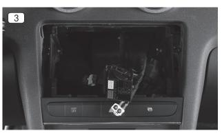
To completely remove the factory radio, all the cables (i.e. main wire harness, antenna cable etc.) must be unplugged on the backside of the device. Put the radio aside in a safe place, to protect it from damage.
