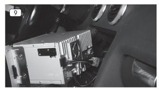
Connect all the cables to the ZENEC system (No. 1) those previously run in the radio slot, and the original antenna cables.
