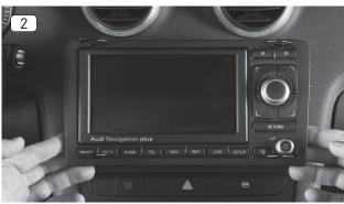
2. It should be possible to pull out the radio without applying brute force.
