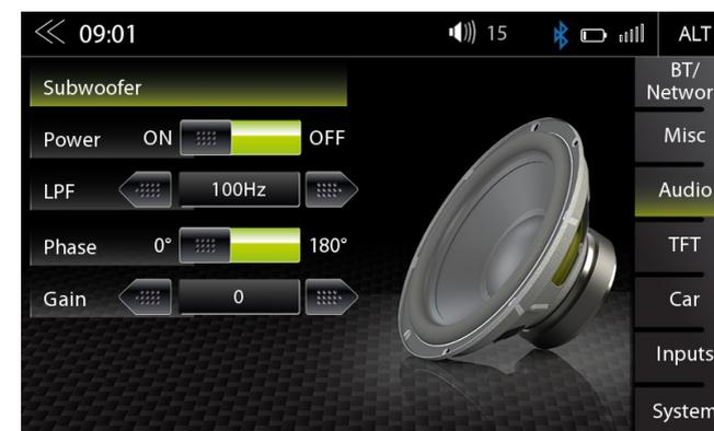
In this Expert Mode menu, you can adjust Phase, Gain, and Low-pass transition frequencies of the subwoofer. The default settings are Phase 0°, Power OFF, LPF OFF.
