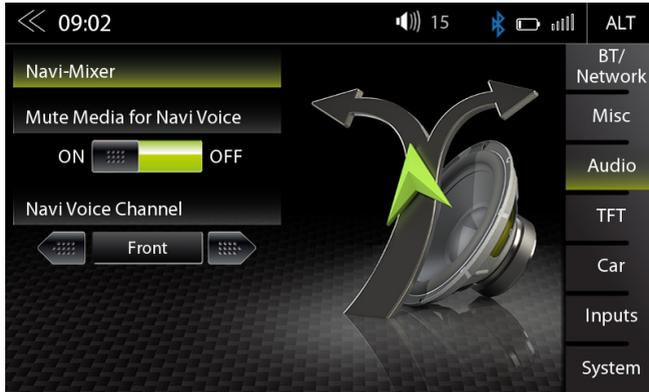
In this Expert Mode menu page, you can adjust audio ducking or mute of audio and video source playback by nav route guidance voice. Secondly, you can adjust if the route guidance voice will be transmitted only via the left front speaker (driver side) or via both front speakers. Works only for ZENEC navigation software.
