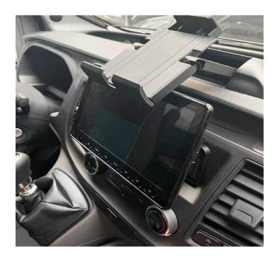
If the radio is replaced with a navigation system with a larger screen, the tablet holder can no longer be opened or will hit the edge of the screen when opened from above.
